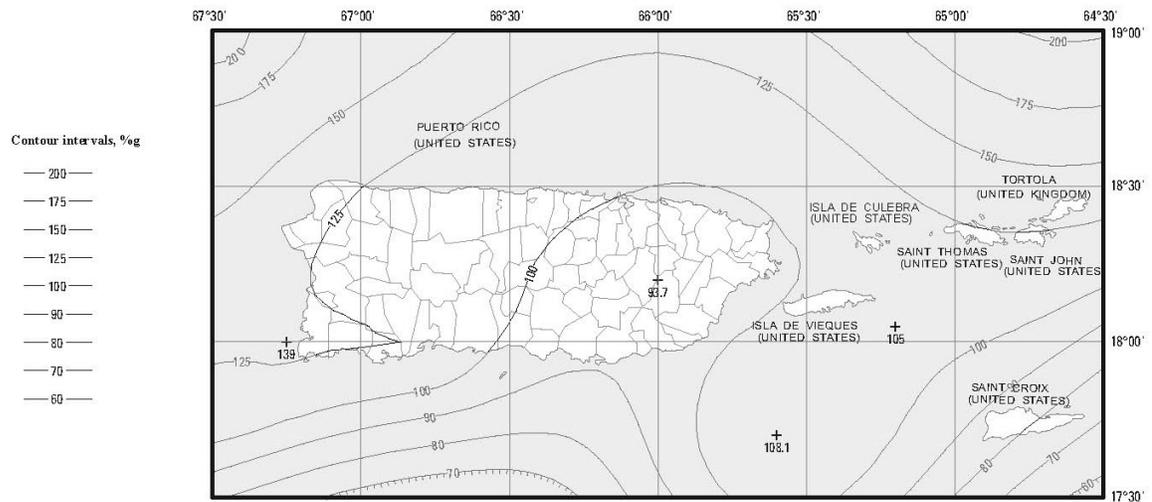
0.2 Second Spectral Response Acceleration (5% of Critical Damping)
