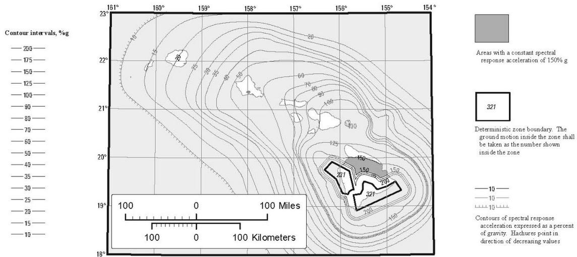
0.2 Second Spectral Response Acceleration (5% of Critical Damping)
