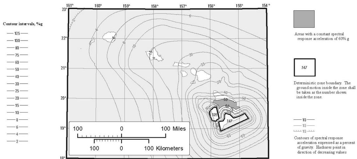
1.0 Second Spectral Response Acceleration (5% of Critical Damping)
