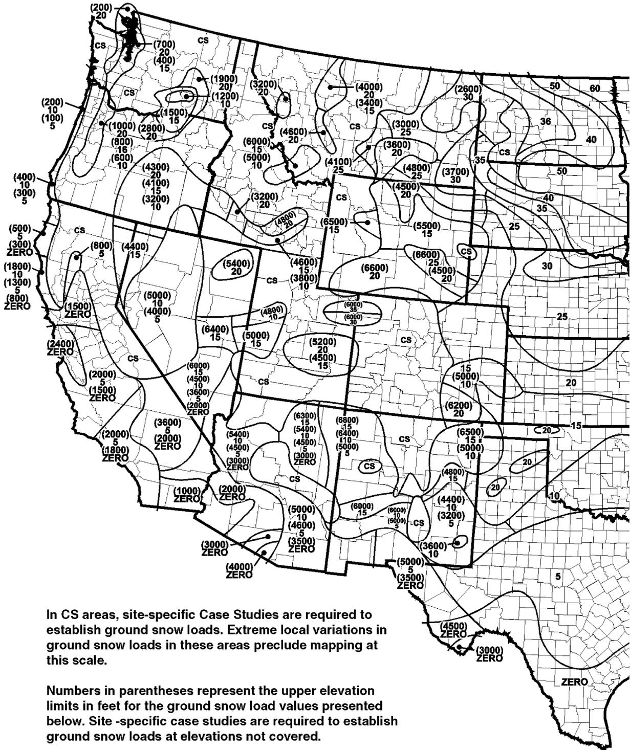
In CS areas, site-specific Case Studies are required to establish ground snow loads. Extreme local variations in ground snow loads in these areas preclude mapping at this scale.
