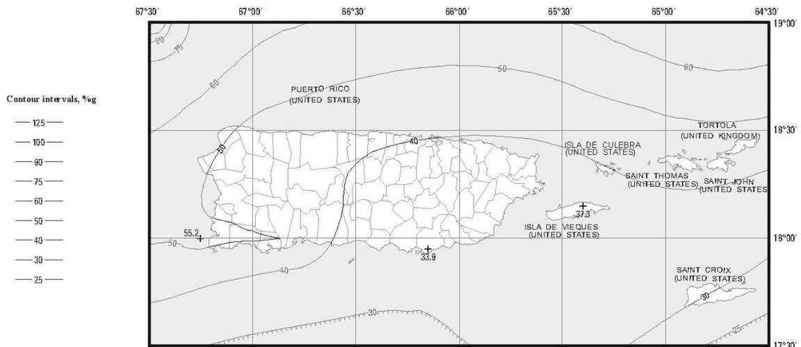
1.0 Second Spectral Response Acceleration (5% of Critical Damping)
